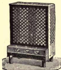
Fig. 185.—Extra Series Resistance for the Moving-Coil Circuit of Wattmeter
